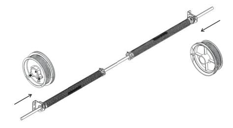
At the end of horizontal rails fasten the torsion springs system.
