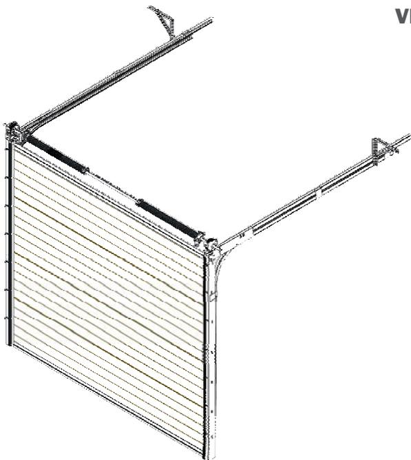
Company Kružík s.r.o. has developed the complete set of track system for sectional doors of residential buildings. It was specially developed for the situations with a headroom of min. 230mm.
